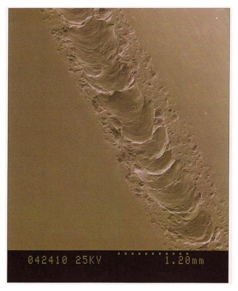
SEM image of the spalling observed on the inside surface of the outer raceway. Magnification 37.5X.
