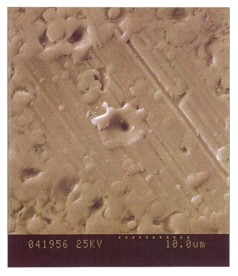
High magnification SEM view of particles flattened onto drive end outer raceway running surface showing variety of particle sizes. Material has clearly been molten at the time of deposit. Magnification 4,500X.
