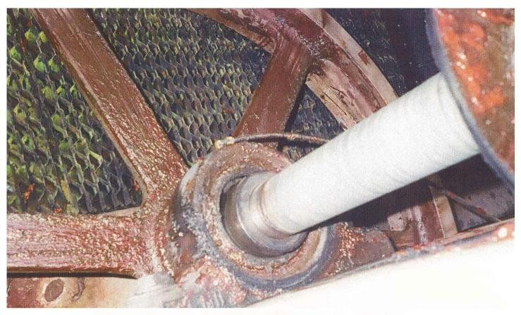
This cooling tower fan drive end bearing failed within two years of running time. The cause was determined to be moisture contamination.
