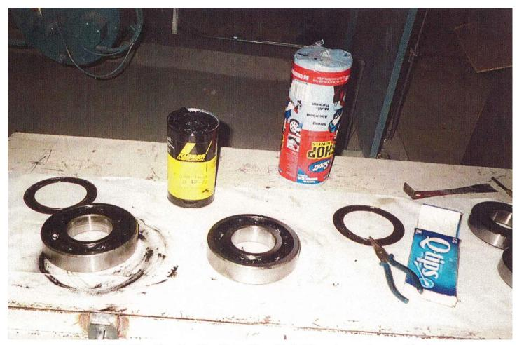
"EIBD" – One Solution Applied = Use Sealed Bearings, clean out factory grease and pack with Electro conductive Grease.
