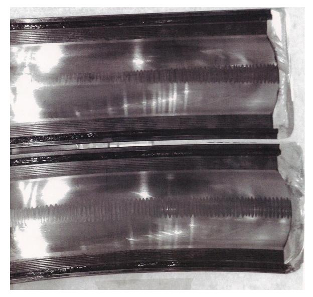
The bearing race shown in this photo was found in the advanced stage of fluting. See scanning electron microscope (SEM) images for the above bearing race on pages 28 and 29.
