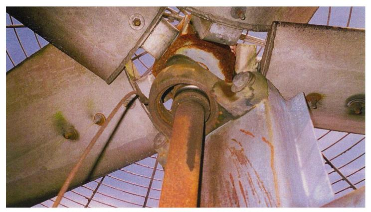
This cooling tower fan opposite end bearing failed within eight years of running time. The causes are cage failure, lack of lubrication or moisture contamination.
