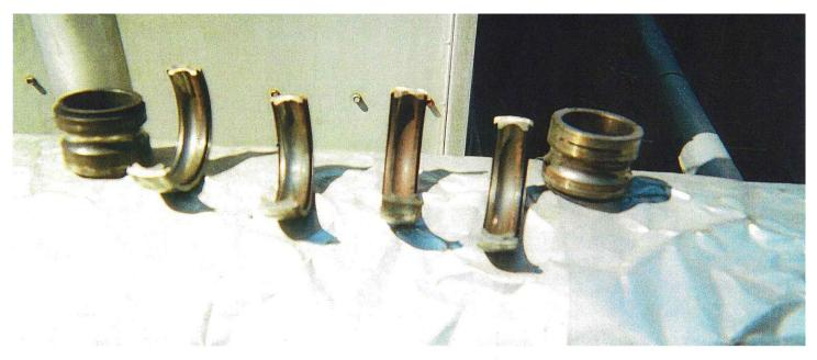
These bearing parts were cut in half to show moisture contamination in a vertical shaft cooling tower. The average life span of new fan bearings on this site is only three years.
