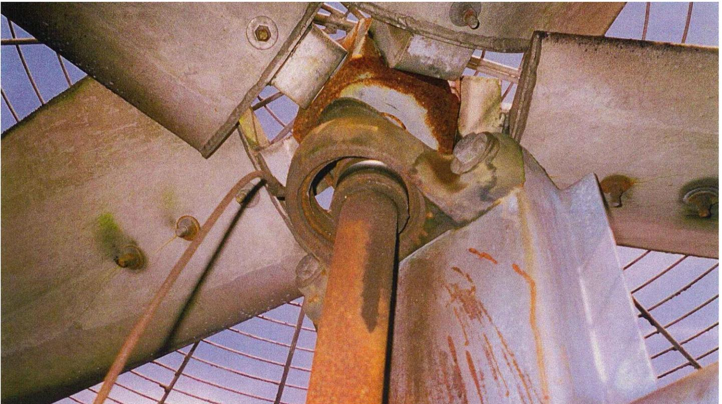
**This cooling tower fan opposite end bearing failed within eight years of running time. The causes are cage failure, lack of lubrication or moisture contamination.**
