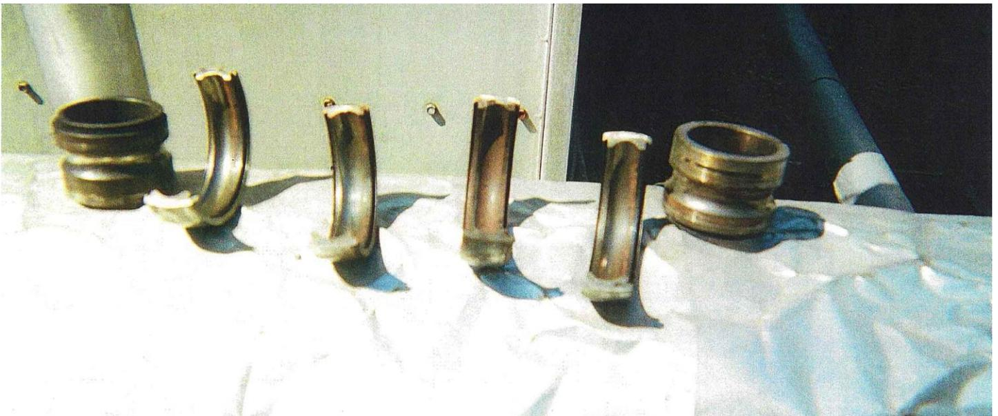
**These bearing parts were cut in half to show moisture contamination in a vertical shaft cooling tower. The average life span of new fan bearings on this site is only three years.**
