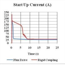
Start-up current for a 25 HP rated coupling
