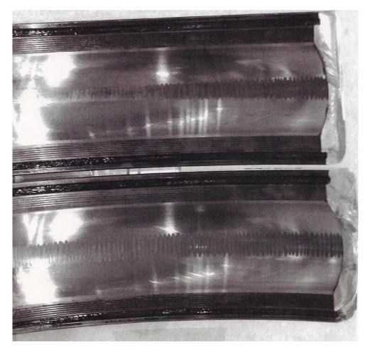
Figure 4: The bearing race shown in this photo was found in the advanced stage of fluting. Vibration spectrum data for this bearing can be reviewed on pages 16 – 19. See scanning electron microscope (SEM) images for the above bearing race on pages 14 and 15.
