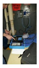
Figure 4 = 10 HP VFD / Junction Box (Typical Rogowski Coil -Electrical Discharge Testing) -AHU
