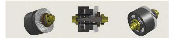
VARIABLE SPEED WITH NO PERIPHERAL COST > EQUIPMENT PROTECTION. NO HARMONICS. Adjustable speed is achieved by controlling the overlap of the Can and Rotor. As the Can and Rotor are disengaged, the slip increases allowing the output speed to decrease proportionally.
