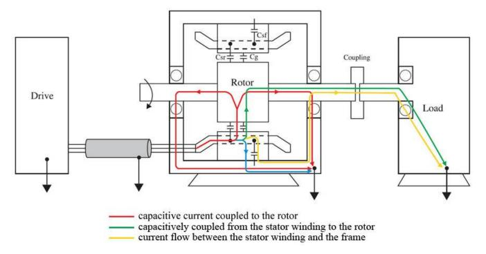
Figure 3: Common bearing current paths in an inverter-driven motor system
