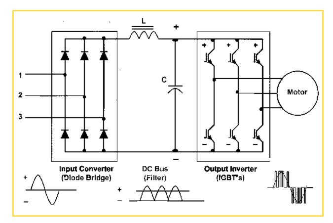
Figure 12: PWM Adjustable Speed Drive Inverters
