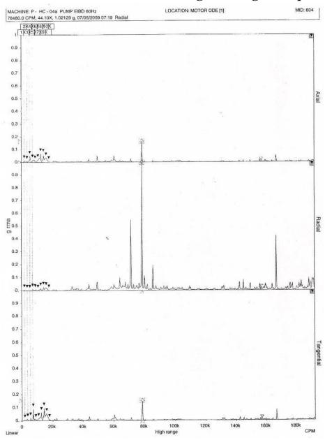
Figure 10: Electrically Induced Bearing Damage @ 60 Hz. The vibration spectrum data shown above was recorded from the bearing (photo) on page 12.
