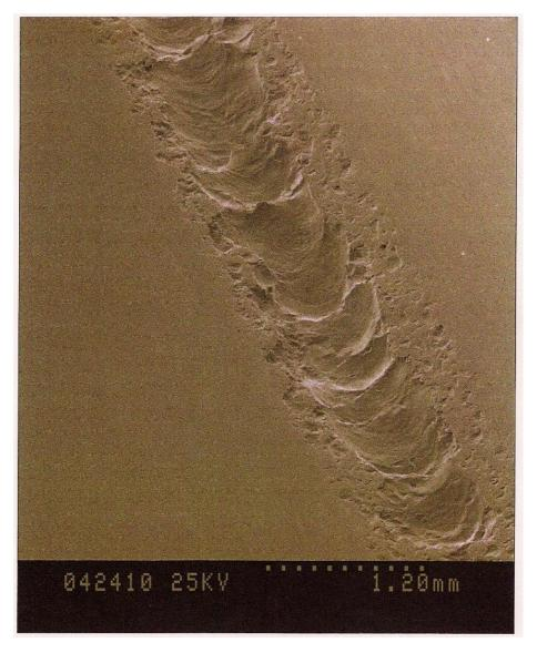
Figure 7: SEM image of the spalling observed on the inside surface of the outer raceway. Magnification 37.5X.
