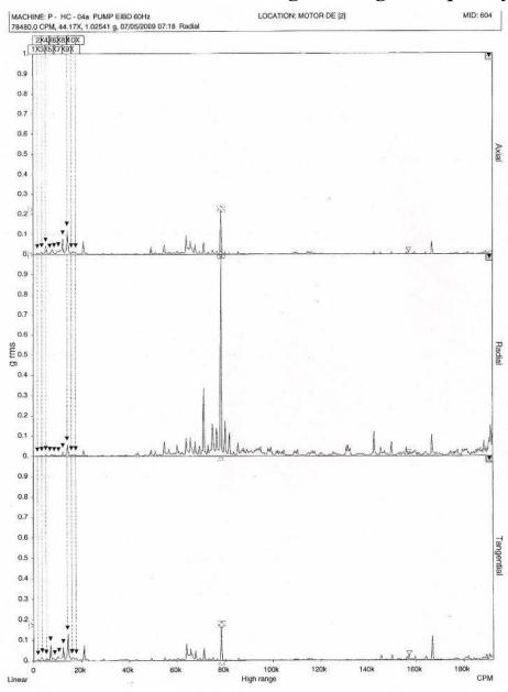
Figure 11: Electrically Induced Bearing Damage @ 60 Hz. The vibration spectrum data shown above was recorded from the bearing (photo) on page 12.
