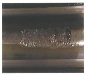
Figure 5: These two photos of the same bearing outer raceway show advanced shaft current / electrically induced bearing damage just prior to failure. Taken September 2011.
