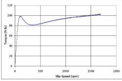
Speed / torque characteristics of a 25 HP rated Flux Drive® ASD
