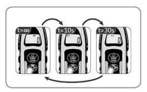
6. If the measuring time selected is infinite: press the start/stop button once to begin the measurement, and press the start/stop button once again to stop the measurement:
