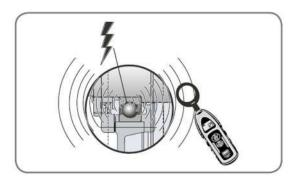
2. Use the TKED 1 as close as possible to the bearing location to perform a detection. Avoid the vicinity of the cables and the Variable Frequency Drive (VFD) controller, which could induce some disturbances:
