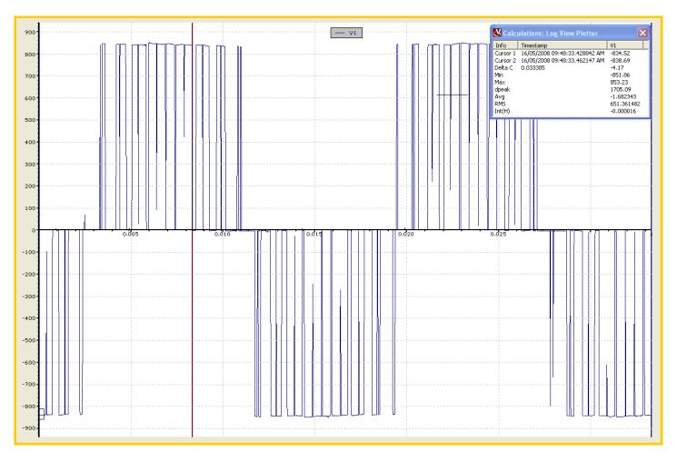
Figure 13: Typical PWM Output Voltage: 600V at 2 kHz
