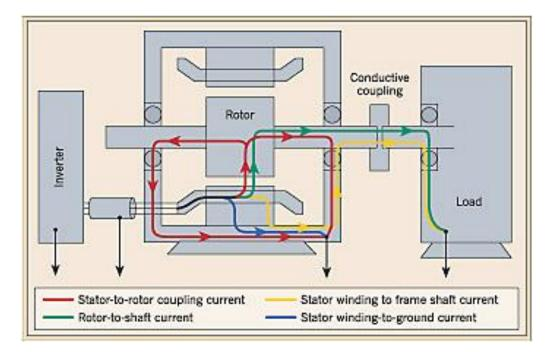
Figure 15: Motor Bearing Currents
