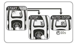
8. If the sampling time selected is 30 seconds: press the start/stop button once to begin the measurement. The measurement will stop after 30 seconds, or if the start/ stop button is pressed again:
