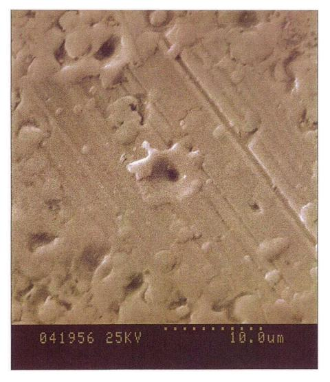
Figure 6: High magnification SEM view of particles flattened onto drive end outer raceway running surface showing variety of particle sizes. Material has clearly been molten at the time of deposit. Magnification 4,500X.
