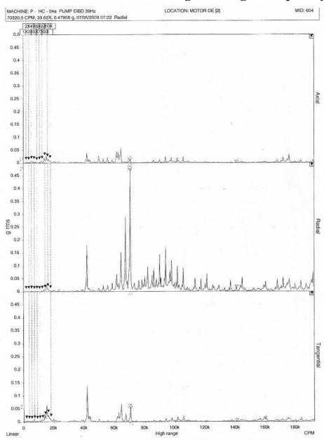
Figure 9: Electrically Induced Bearing Damage @ 39 Hz. The vibration spectrum data shown above was recorded from the bearing (photo) on page 12.
