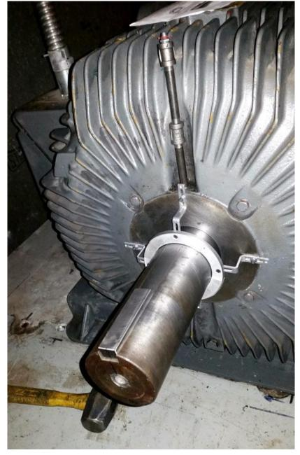
AEGIS SGR SEAL INSTALLED ON A MOTOR DRIVE END
