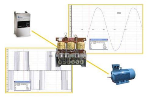
Figure 17: INVERSINE AUSF Performance (Voltage)
