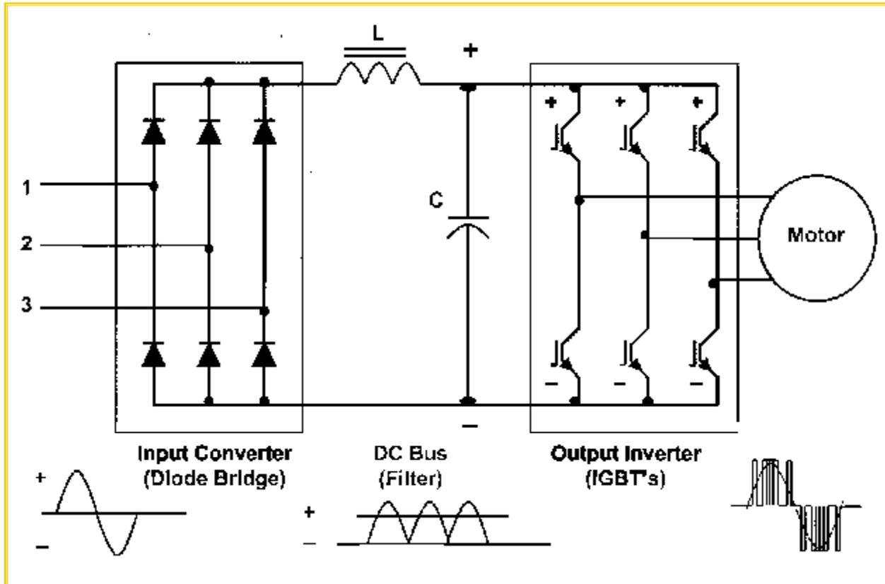
Figure 12: PWM Adjustable Speed Drive Inverters
