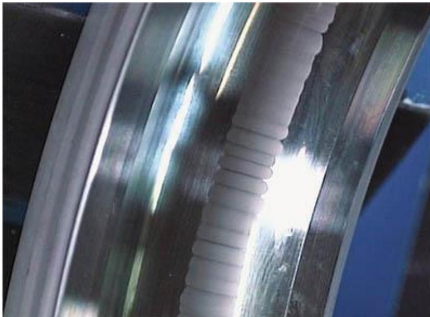
Figure 2: Fluting pattern in an outer bearing race. Vibration levels for the bearing of a motor that is experiencing these defects due to EIBD can be seen on pages 16 – 19.
