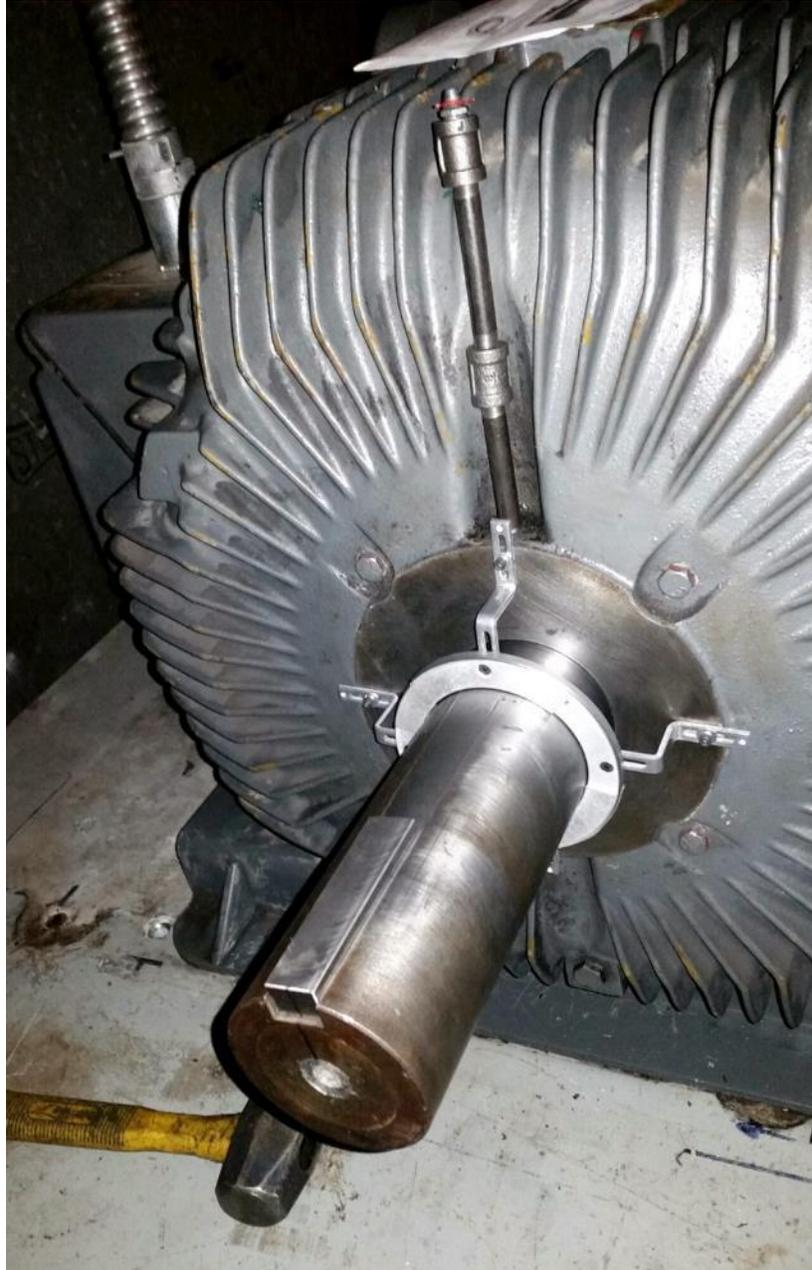
AEGIS SGR SEAL INSTALLED ON A MOTOR DRIVE END
