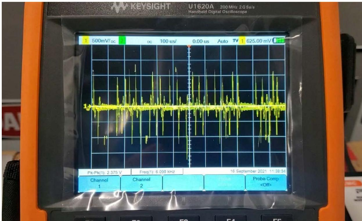
*Electrical discharge levels seen on an Oscilloscope using Rogowski Coil helps determine potential shaft current issues*
