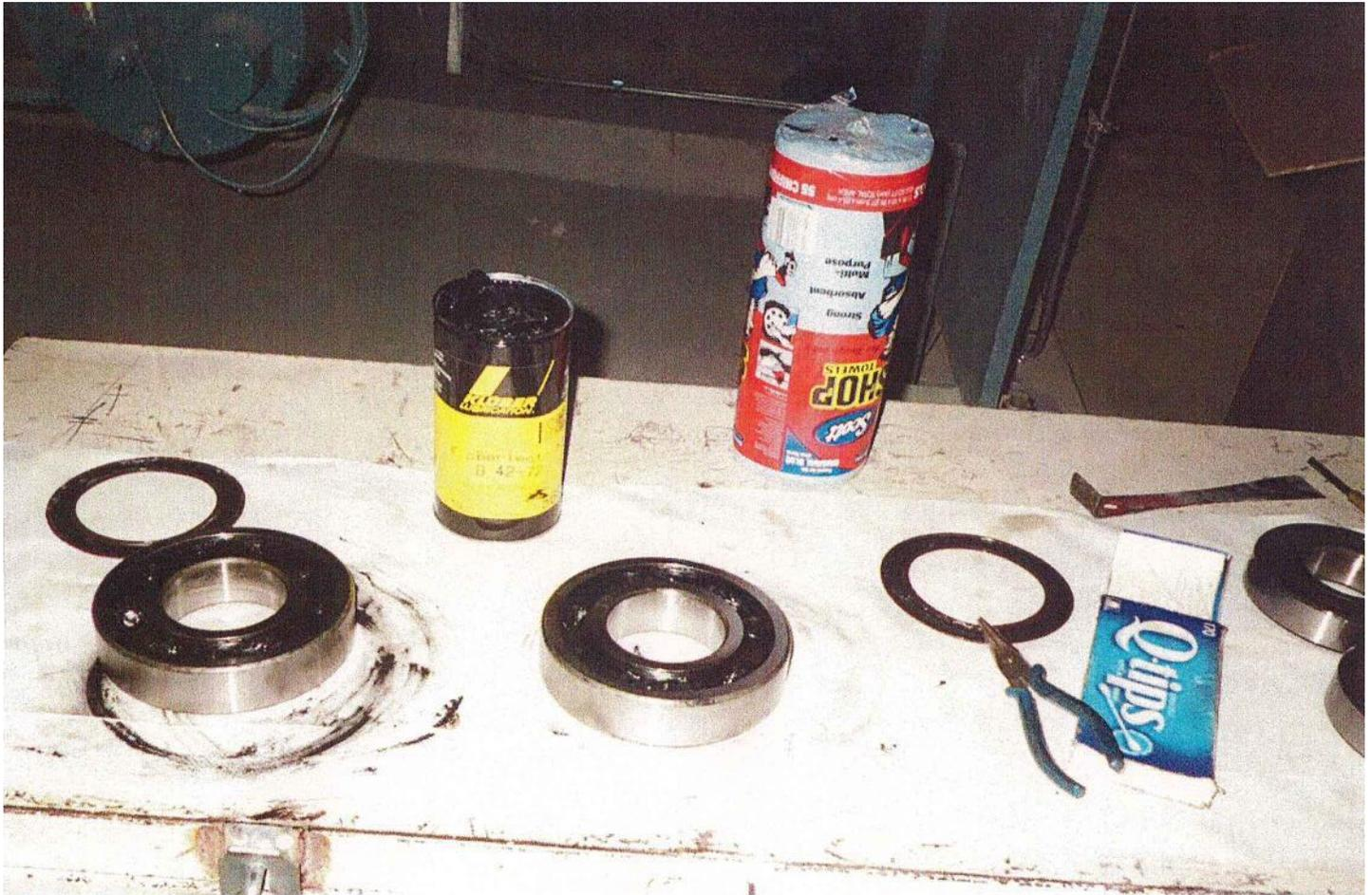
**“EIBD” – One Solution Applied = Use Sealed Bearings, clean out factory grease and pack with Electro conductive Grease.**
