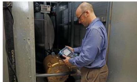
Test Motors with AEGIS® Shaft Voltage Tester® Oscilloscope
