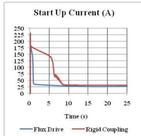
Start-up current for a 25 HP rated coupling
