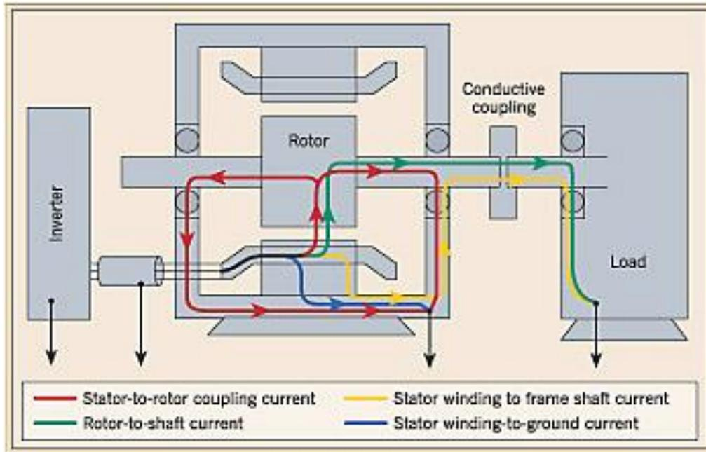
Figure 15: Motor Bearing Currents
